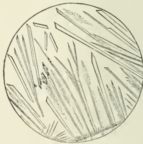
Prismatic Crystals of Corrosive Sublimate from a solution in water, magnified 30 diameters.
